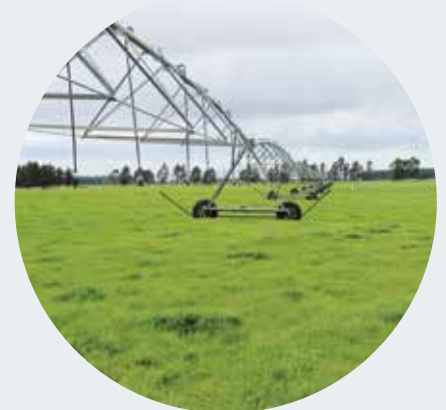
This pivot irrigates and provides fertiliser for pasture through a fertigation system.
