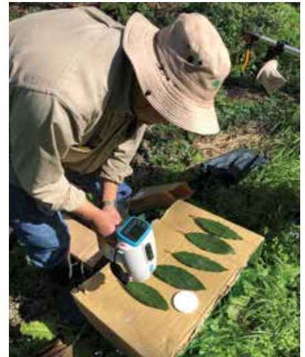
Radiometric in-field measurement of avocado leaves to estimate mineral status of avocado trees and fruits
